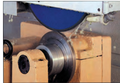
Dia. 2. Method of Dressing for Each Type of Diamond and cBN Wheel
