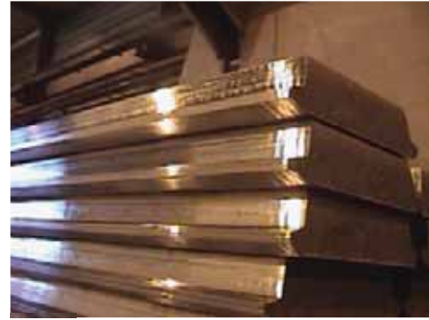
Machined Component: Heat Exchanger panels / Weld Prep
