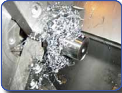
Chip jamming during outer machining
