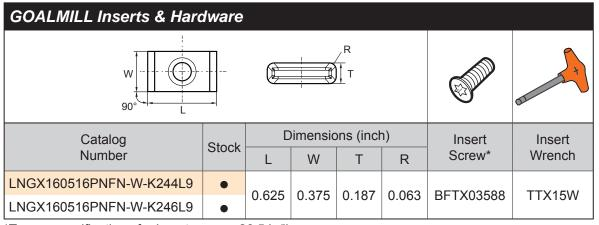
\*Torque specifications for insert screw= 26.5 in/lbs.
