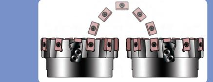
By switching the insert to a left hand cutter, FOUR MORE ROUGHING EDGES can now be used. A total of 12 indexes are possible when using both right and left hand cutters.\*
